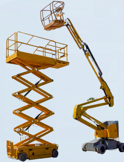
Boom Lift & Scissor Lift
